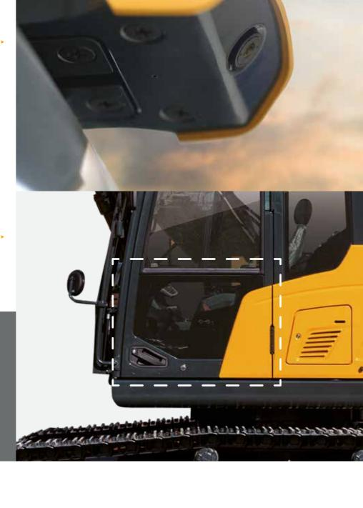
The auto safety lock feature prevents unintentional ignition. While the auto safety lock is activated, the excavator is not controlled by the RCV lever.
